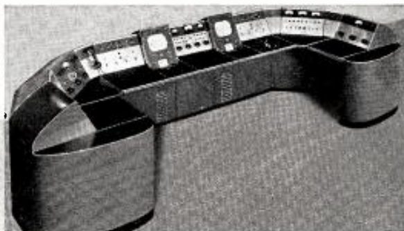
De luxe set-up for combined centralized control . . . AM-FM and TV. Extreme left and right sections are the AM (or FM) transmitter controls. Each includes a transmitter-control, audio-control, and blank wing turret. Center turret controls (for RCA 5-kw TV transmitter) are, left to right: TV power, picture monitor, TV audio, preview monitor, TV program switching.
